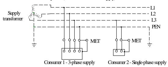
In a TN-C-S system the neutral and protective functions are combined (C) in a single protective earth and neutral (PEN) conductor in supplier's distribution. The system is also known as a protective multiply earthed (PME) system, as additional earthing, say at every third pole of an overhead supply, guards against a hazard arising from the unlikely event of a broken neutral.
