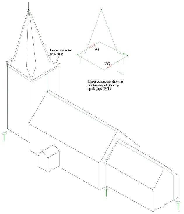
Note: The system layout, including bonding connections, which are not shown here, should facilitate testing as described in 8.2
