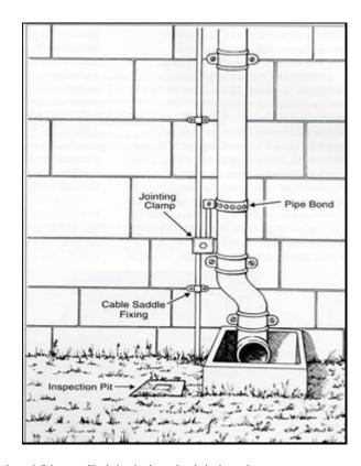
Note: In (b) there normally would be a test break/bi-metallic joint below the jointing clamp
